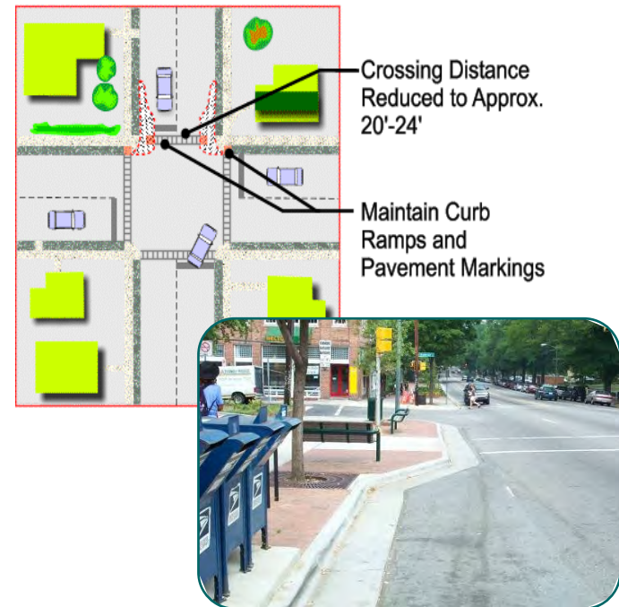
Exhibit 5-10—Example of bulb-out placement to reduce curb radii and shorten crossing distance for pedestrians.
